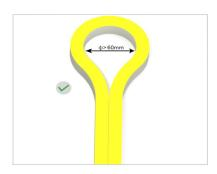
When lighting direction on Side. The vertical bending diameter need to more than 60mm.
