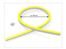
When lighting direction on side. The horizontal bending diameter need to more than 80mm.
